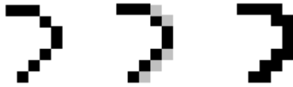
Figure 6: Lines 1 and 3 have been thinned with CC and Zhang-Suen methods, respectively. The central line shows the “difference” between both.
