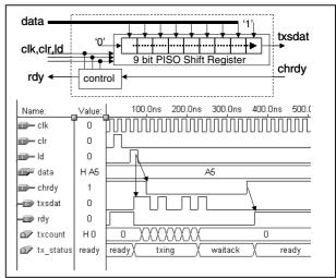
In this serial port, the data frame start bit behaves as the transmitter handshake signal (equivalent to *new* in the parallel port); in this instance *chrdy* is the receiver's response (equivalent to *ack* in the parallel port).
