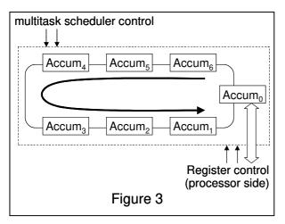
the worst case, if task 0 must be switched to task 6, the context switching latency could be 6 clock cycles.
