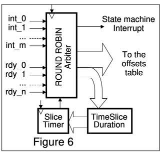
The simplest case is a multitasking system with equal priority tasks, using a "round-robin" arbitration scheme (Figure 6). In this case, the schedule of a new task may have several causes:
