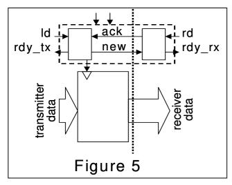
• The other situation is when the receptor is willing to read new data when it is not present (*new* inactive). In that situation the signal *rdy\_rx* remains inactive until the transmitter writes new data.
