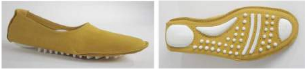
Figure 2: The shoe design – made from 3 materials that are attached to each other only by sewing. The insole - sole is a one-piece 3D printed according to a specific foot.
