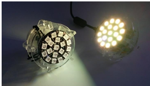
Figure 3. Lighting component design and implementation.
