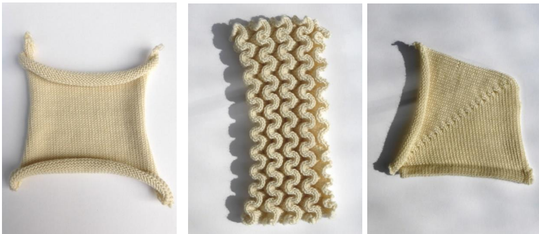
Figure 3 classes of weft knit fabric; plain knit, links/ links and partial knit. source: Scott.
