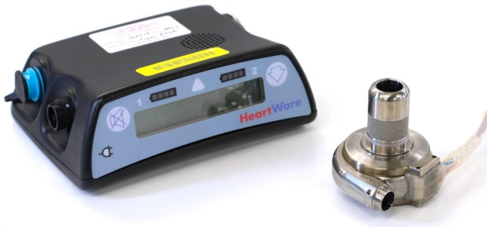
Figure 1 Ventricular Assist Device (VAD) and controller (image taken by author)
