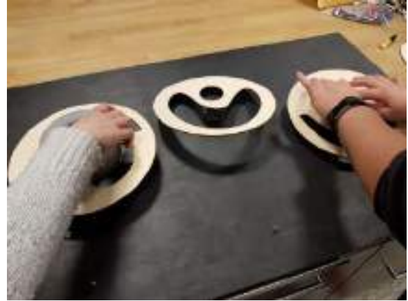
Figure 10: Three related shapes, drawn as vector graphics and cut on a laser cutter at a nearby makerspace. In this case, the students had to adjust their original concept with servos off center and put the shaft as close to the center of gravity as possible.
