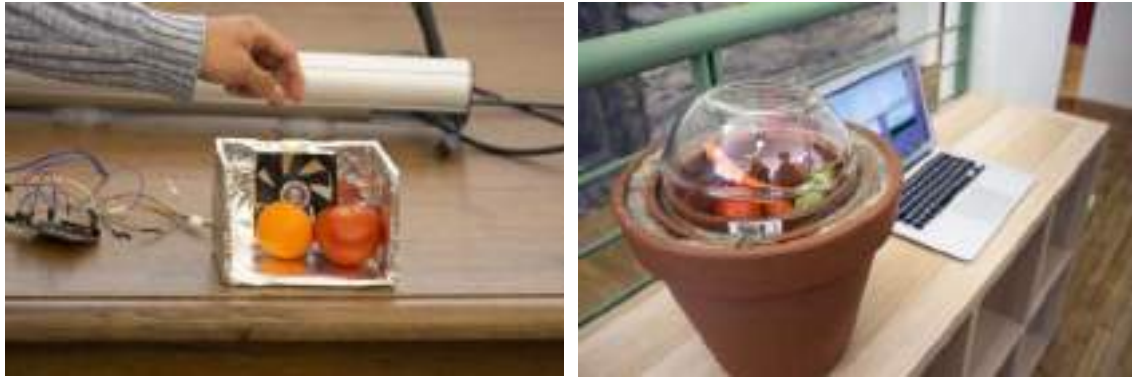
Figure 4: Temperature and humidity monitoring prototypes
