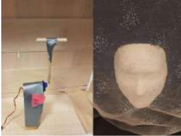
Figure 9a and 9b: The length of an arm (a) had to be a tradeoff between the distance the plaster face (b) could be pushed and the strength of the servo. The weight of the face and the material the face is pushed into, also have to be considered.
