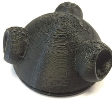
Figure 5. An example of a poor-quality 3D print finish occurring from the layering process on curvaceous surfaces. This is avoided by reorienting the product on the print bed.
