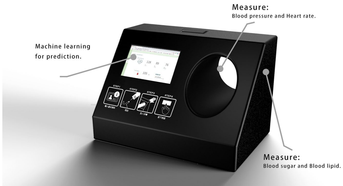
Figure 3.3 Intelligent health care platform 3D model design.
