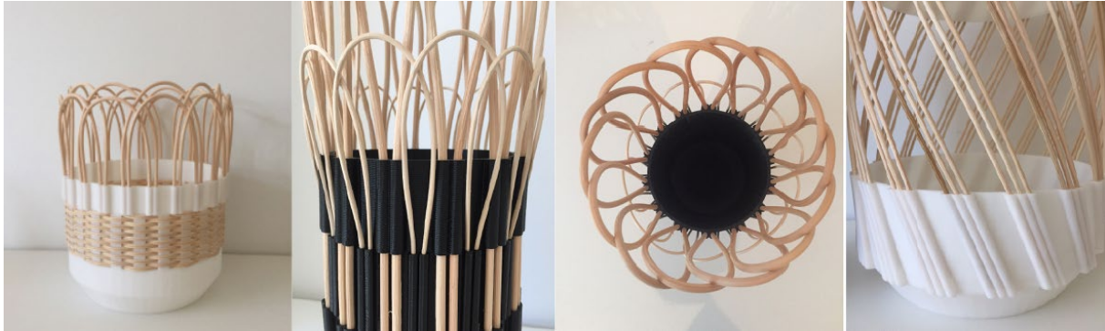
Figure 2 Details of the Hybrid Material Vessels, variations in printed components and rattan weaving.
