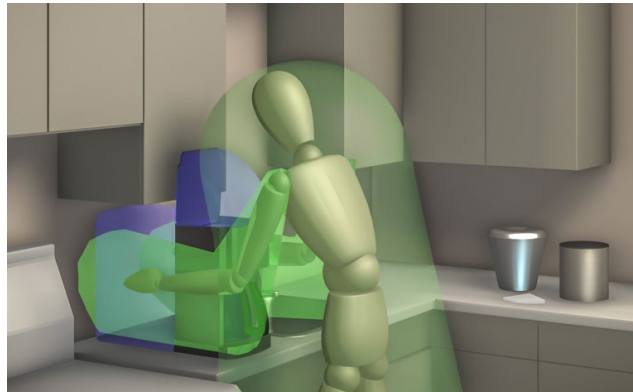
Figure 3 Phantom volume required for the user’s body in relationship to the coffee maker. Note also counter space occupied by the can of fresh coffee, coffee filters, and compost bin.
