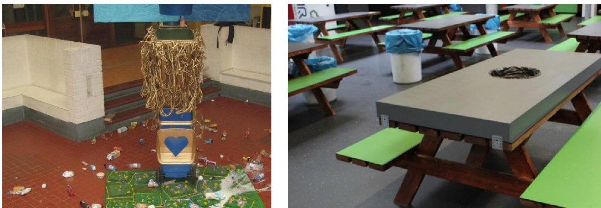
Figure 2 (left) Playful design of a waste bin didn't work (right) Mock-up of the alternative solution with a waste bowl integrated in the middle of the lunch table (de Waard, 2012).
