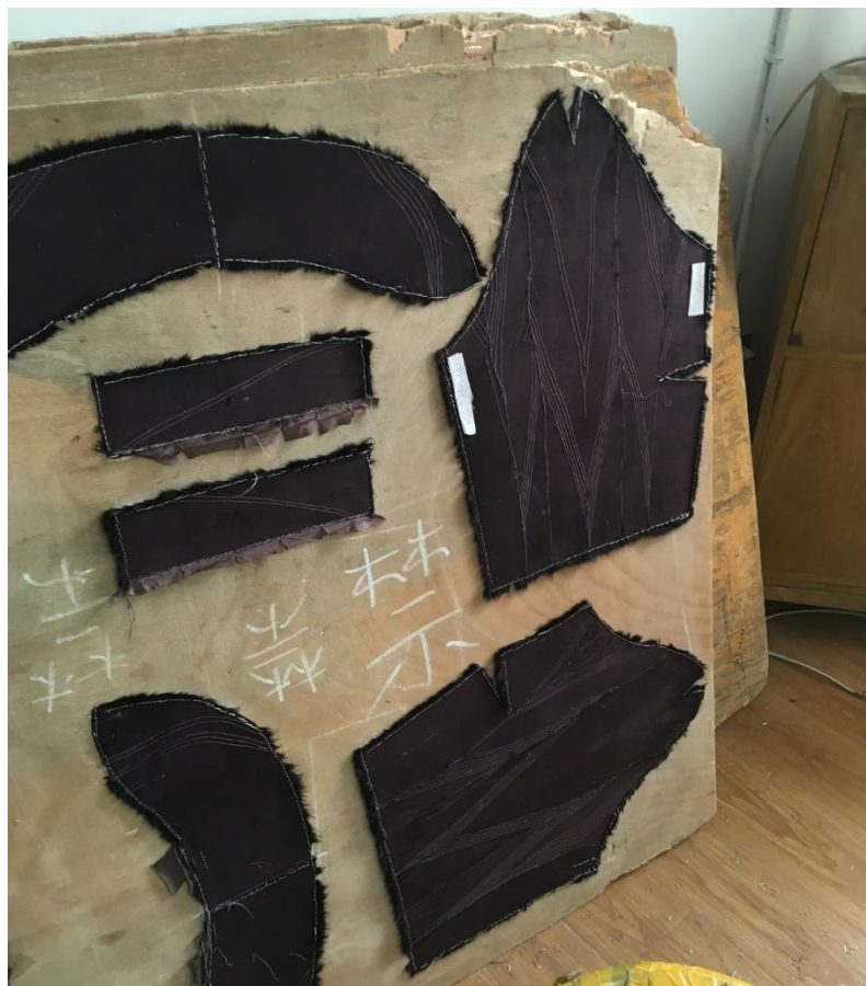
Figure 6: Fur coat that has been disassembled, re-dyed and stretched before being sewn back together.
