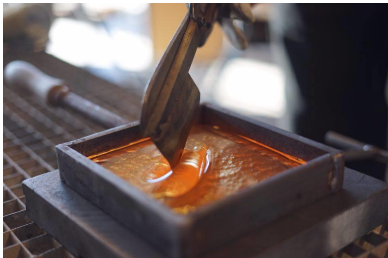
Figure 5 Additional glass shaping to add layered qualities. Source: Mads Hoby
