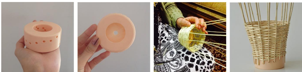
Figure 13. Initial trials with bases produced by a 3D printer
