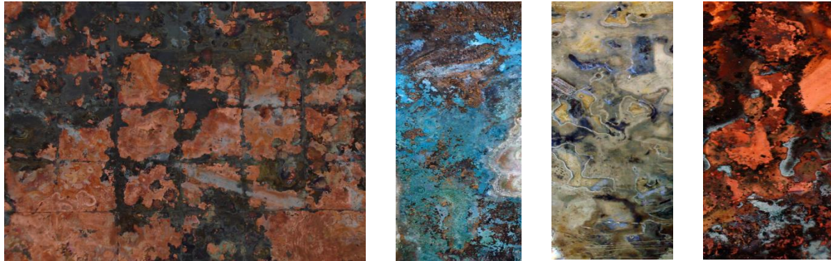
Figure 17, 18 and 19: Microbial patination of metal sheets. Bacterial cultures on test samples, copper and brass sheets. The left sample is 3*5 cm. Photo: Johnsrød. Source: Johnsrød (2009)
