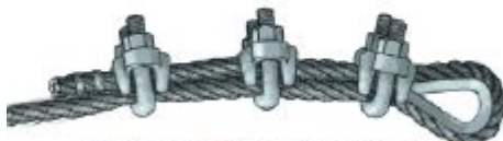
U-Bolt of all clips on live end of rope.
