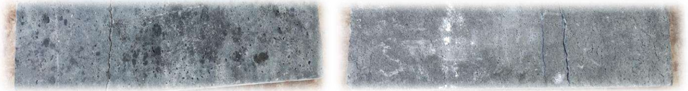
Figure 8. Rupture mechanism of designed samples under flexural loading.
