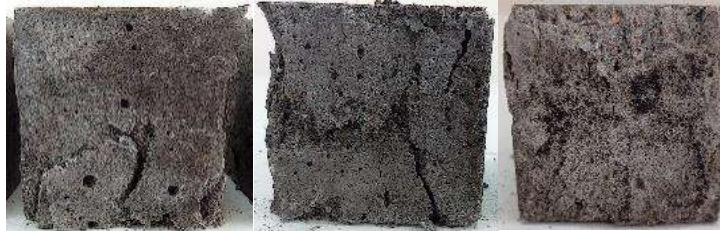
Figure 9. Rupture mechanism of designed samples under axial compression
