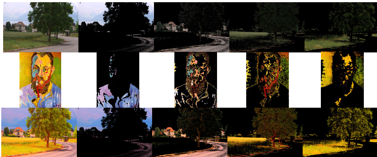
FIGURE 3. Multilevel color transfer using the b^* component. First row exhibits the input image, second and third rows correspond to the target and the outcome, respectively. Left to right: The working image, followed by its four partitions.
